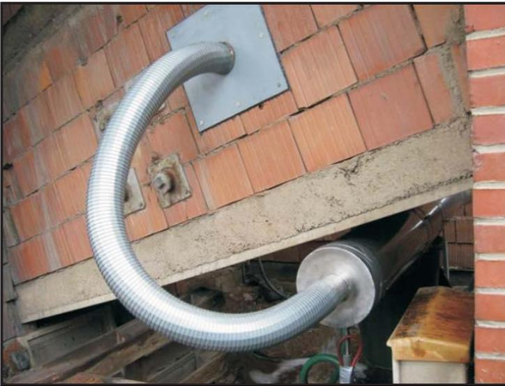
Exhaust air is induced into the test spray tunnel through a flexible metal pipe.
