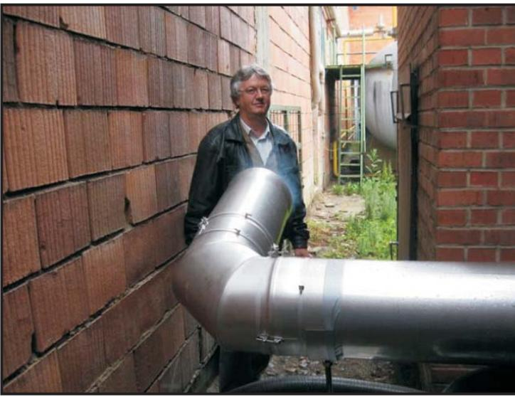
The test facility consists of an exhaust air pipe with built-in spray nozzles and a diameter of 300 mm - 11.8 inches - set on pedestals and a droplet separator, a spray water pump, and a spray water container.
