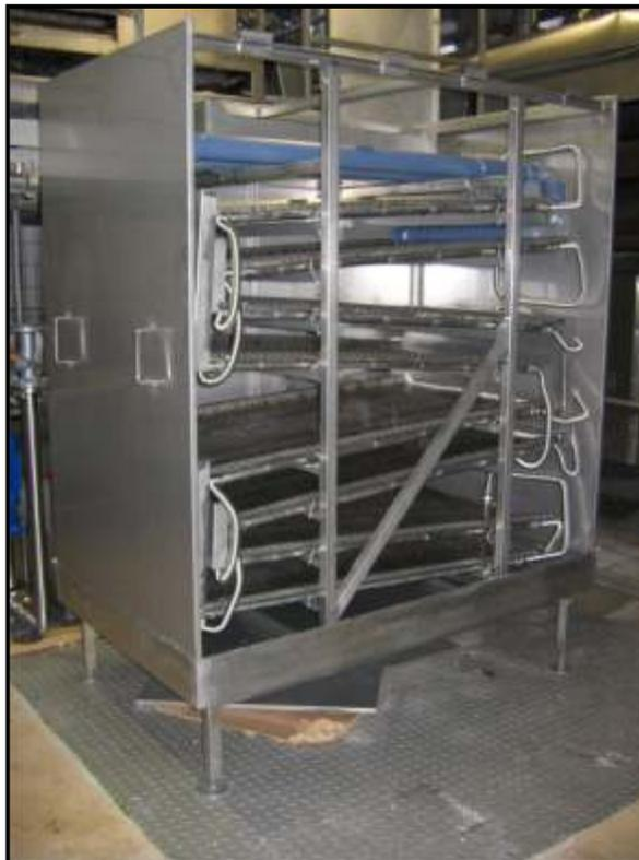
Photo: FERCHER Wastewater Heat Exchanger Type FB-8/S, before start-up.
